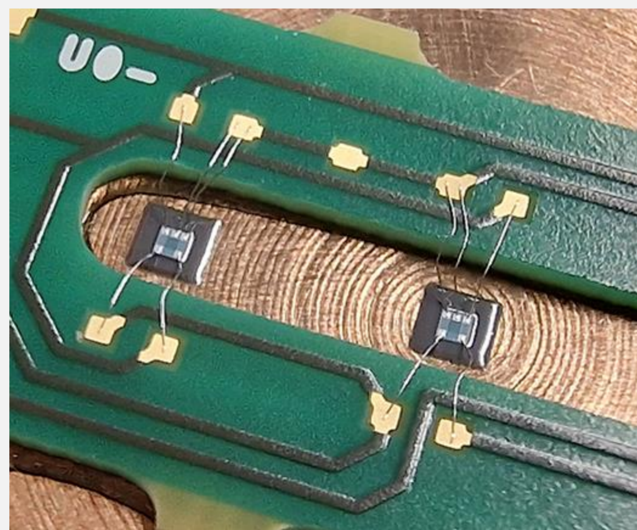
Two distributed sensors mounted on the screw head to correct measurement errors in the event of inclined loads
